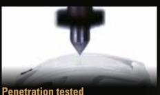
All Arai helmets are penetration tested, (except Freeway-2, Penta, Astro-Light and VX-Pro Jr) although not required by European helmet standards. The Arai penetration test is performed with a 3kg test cone that strikes from a height of 3m on the helmet.
